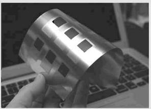
The rechargeable battery contains a vanadium-oxide cathode, grown on a sheet of graphene paper, an unidentified separator, and an anode made of lithium-coated graphene.
